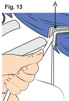
5. Make sure the patient's lower back is positioned all the way in against the chair/wheelchair and that the weight of the patient is taken up by the receiving surface before unlocking the cords from the cleats (A). (See Fig. 13)
