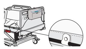
Place the power cable in the cable management loops on the left side of the bottom mattress cover. Secure the cable using the six cable loops with locking clips.
