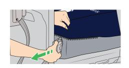
For Reactive therapy disconnect the pump tube-set connector.
