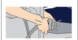
For Active (alternating) therapy connect the pump tube-set connector, make sure it clicks into place on both sides (double-click).
