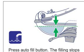
automatically at correct water level.
