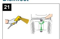
Spray disinfectant in the drain. Close the drain.
