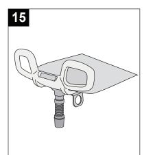
Spray disinfectant on upper drainage and clean with a bottle brush.
