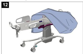
Place disinfected backside of mattress over disinfected head panel and side supports. Non-disinfected inside of mattress facing up. Push out mattress corner creases.
