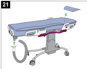
Attach lower drainage to upper drainage and place pillow on mattress.
