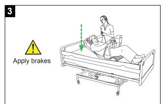
Apply the central brake on the lift bath trolley. Lower the lift bath trolley onto the bed. Lower the backrest until the stretcher is flat.
