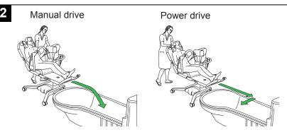
With manual drive: Move the patient over the bath. With power drive: Activate power drive and move the patient along the side of the bath. Push the lift bath trolley sideways over the bathtub.
