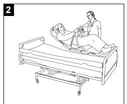
Adjust the lift bath trolley height and move it as far as possible over the bed.
