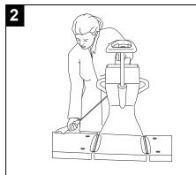
Fasten the hook rope to the side of the lift bath trolley that will function as backrest.
