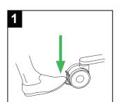
Apply the brakes on the bed, if applicable. Fold down the bed rail on the caregiver side.
