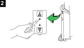
Insert thin, blunt object into the hole and press to raise or lower the lift bath trolley.
