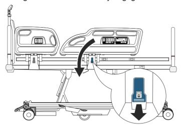
Pull the blue release lever to lower the side rail.
