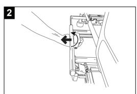
Squeeze extension latch to unlock and pull section until fully extended.
