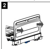
Pull out the bed frame to required position and release handle.
