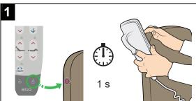
Hold the magnetic sensor over a magnet for 1 second.
