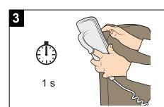
To exit, hold the magnetic sensor over a magnet for 1 second.
