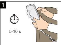
Hold the magnetic sensor over a magnet for 5 to 10 seconds until there is a beep.
