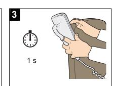
To exit, hold the magnetic sensor over magnet for 1 second.
