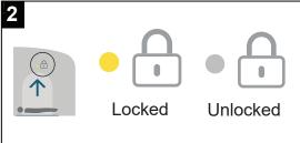
Press the function buttons to lock or unlock each function.
