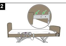
Pull the footboard to the desired length as marked on the bracket. Tighten the screws on both sides.
