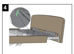
Put down the mattress platform extension over the stopper to lock the position.
