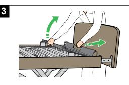
Lift the plastic end of the mattress platform extension and pull the metal frame to the same length as the footboard.
